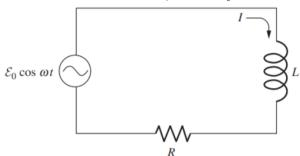
The Kirchhoff loop equation for the series RL circuit and the alternating current is
