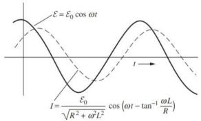
Since  $\phi$  is a negative angle, the current reaches its maximum a bit later than the electromotive force.
