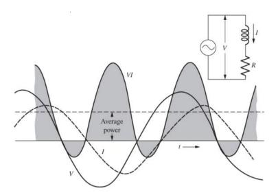
(2) The average power  $\bar{P}$  delivered to the RL circuit corresponds to the horizontal dashed line.
